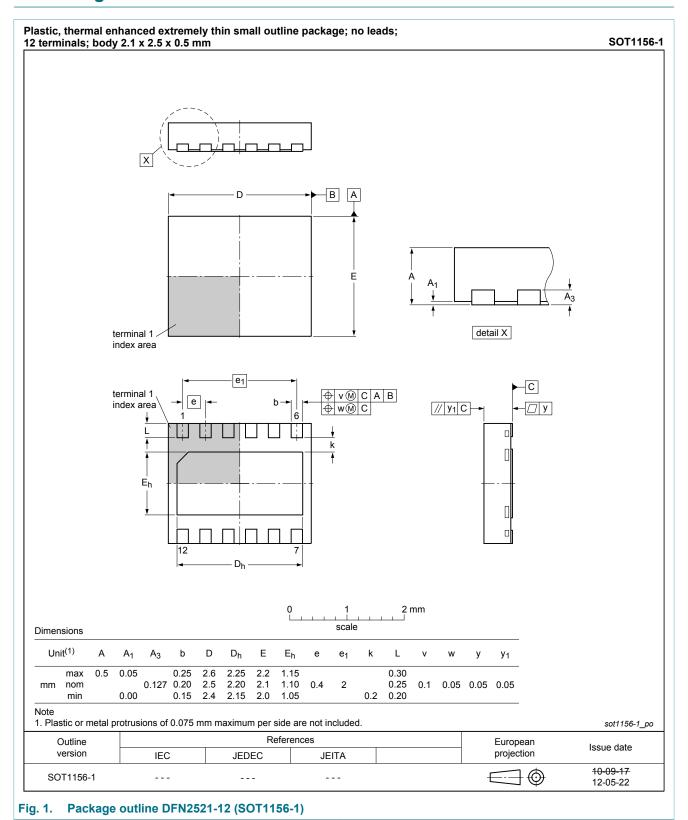
plastic, thermal enhanced extremely thin small outline package; 12 terminals; 0.4 mm pitch; 2.5 mm x 2.1 mm x 0.5 mm body
